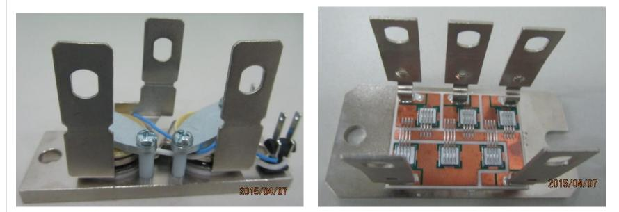
With the help of the opened samples, the differences between pressure contact and solder contact modules can be clearly displayed. The higher reliability oft he pressure contact modules can be made visible.
